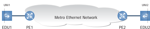
Figure 1. Both operator and the customer can initiate loop-back to the remote demarcation point to verify the status of the connection.
