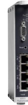
Fig. 4 TS-Series Node Management Board (NMB) handling all plug-in units in the TS-Series
