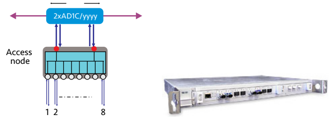
Fig. 3 An example of the compact and low power consuming configuration of a TM-101 chassis
